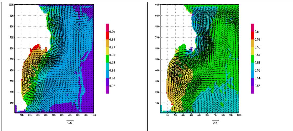
**Fig. 10 - Results of the coastal model: sea level elevations (shaded, in m) and currents (vectors, in m/s), for processing of tides and winds from southeast (left) and tides and winds from northeast (right).**
