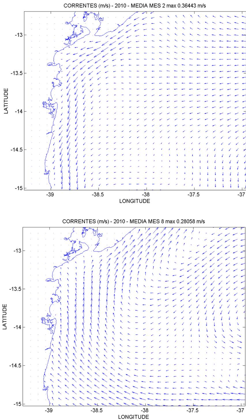
**Fig. 9 – Monthly mean surface currents, computed by Hycom numerical model, in February and August 2010 ( <http://www.hycom.org/> ).**
