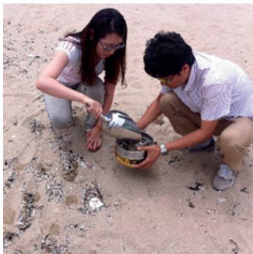
Figure 3.5 Collecting microplastics from surface sediments by dry sieving, prior to carrying out compositional analysis; Busan, Republic of Korea.
