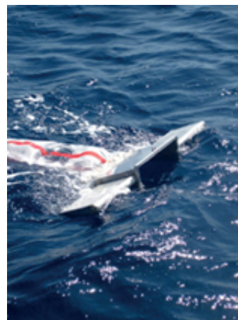
Figure 3.4 Manta net being used to collect microplastics from surface waters in the Pacific, operated from S/V Kaisei, 2009. Image courtesy of Doug Woodring, Project Kaisei; http://projectkaisei.wordpress.com/the-science-team/ .
